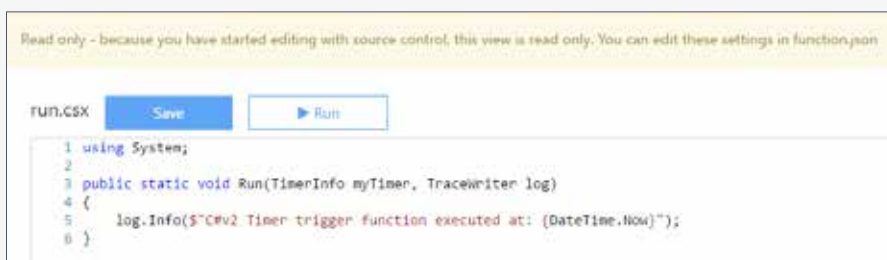
An Azure function becomes read only after configuring source control integration.
